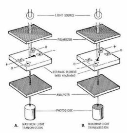
CERAMIC POLARIZATION is changed in the fine-grained ceramic (binary mode) memory element by applying current to various combinations of electrodes —only two of which are indicated in this simplified and enlarged diagram. When the polarization of the polarizer and analyzer differ by 90 degrees as indicated, the extent of light transmission will be determined by the polarization of the ceramic element. Multistate memory is created by switching arrays of electrodes on both faces of the ceramic.
